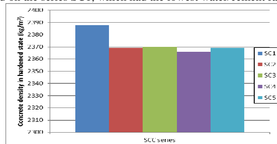
Figure 3: Hardened SCC density at 28 days
