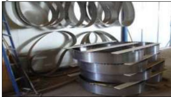
PICTURE 1- bend saw blade-blade of unalloyed or low-alloy steel
