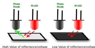
Fig. 5. The principle of sending and receiving light
