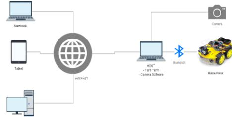
Fig. 9. Remote communication scheme
