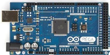
Fig. 2. The Arduino Mega 2560 microcontroller board
