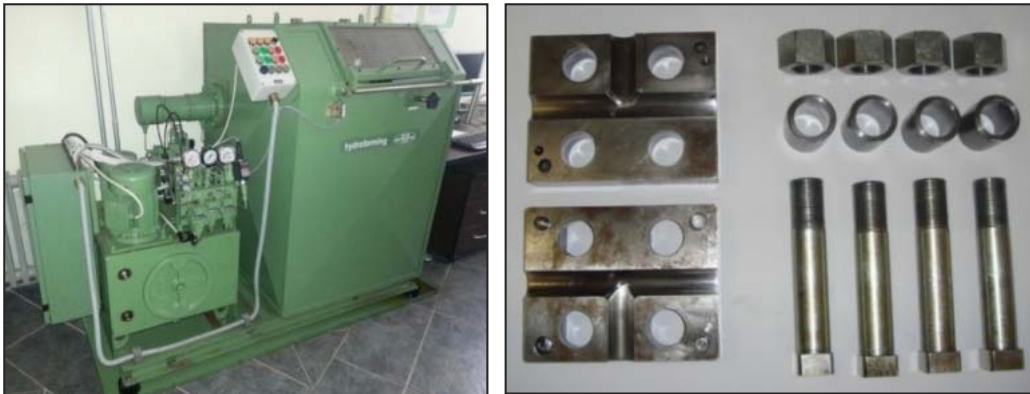
Fig. 2 - A machine and tool for T-shape hydroforming
