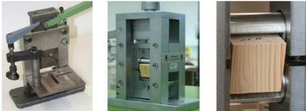
*Figure 9: EN 392 type shearing tool (left), new test apparatus (center), close view of a specimen during testing with the new apparatus (right)*
