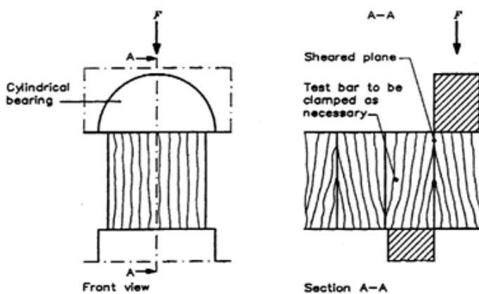
Figure 7: EN392 method of applying shear stress to a glue line
