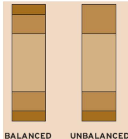
*Figure 6 . Balanced and unbalanced beam*
