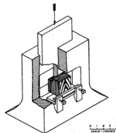
Figure 8: ASTM D 905-03 shearing test equipment
