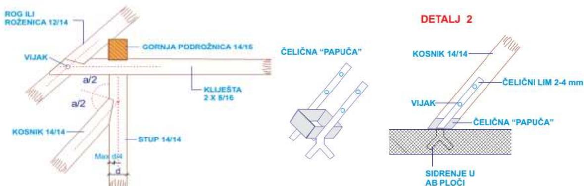
Queen truss can have a range between 7-12m. The minimal gradient is 25°-30° and maximal length of rafter is 7-7.5m.
